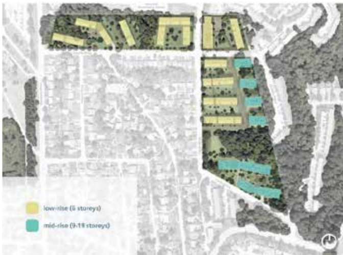
Figure 12: Building Forms (note: at the mid-rise zones, the number of storeys increases on the downhill slope where ground-orientated floor levels are each counted as a separate storey)
