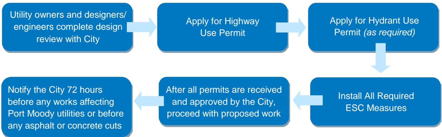
Figure 3: Acceptance & Permitting Procedure for Third Party Utility Construction
